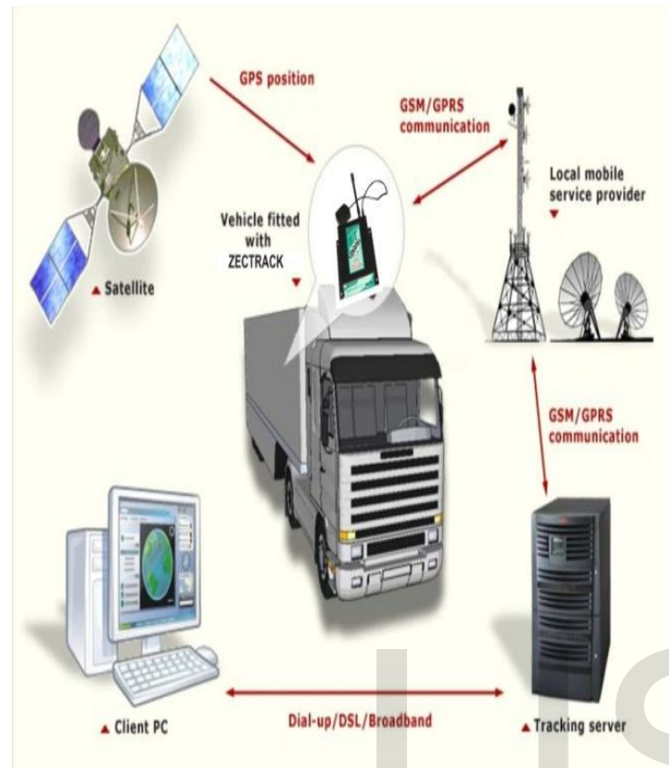
Fig 2.1 GPS SYSTEM INSTALLING [2]
